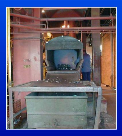
Castings proceed through shakeout to remove loose sand and coating
